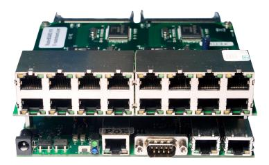
The new RB604 is an expansion board for RouterBOARD 800 and also the RouterBOARD 600 series. It attaches to the RouterBoard device to add 16 additional 10/100 ethernet ports.
