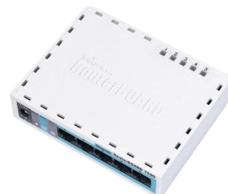
The RB750G is a small SOHO router in a nice plastic case. It has five independent Gigabit ethernet ports and optional Switch Chip functionality for wire speed Gigabit throughput.
