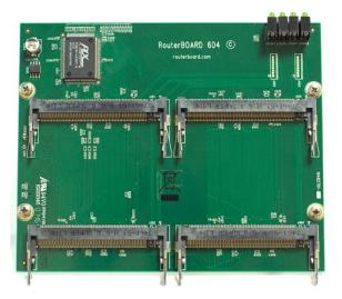
The new RB604 is an expansion for RouterBOARD 600 and also the RouterBOARD 500 series. It attaches to the RB device to add 4 additional miniPCI slots, your RouterBOARD 600 can now have 8 miniPCI slots total!
