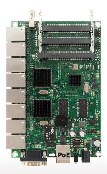
The RB493G has nine Gigabit ethernet ports, three miniPCI slots, and a switch chip, so the ethernet ports of your choice can be grouped together to make it act as a switch.
