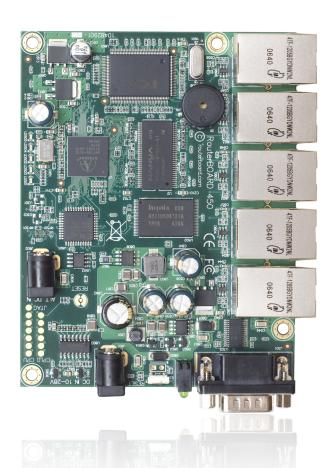
The rb450 is a five port ethernet router. The rb450 is replacing rb150, but introduces at least three times better thoughput.
