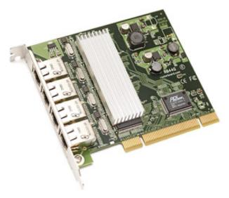
This is the perfect four port card for a router or a server. The easy to use MDI/X feature (accepts both cross-over and straight cables) can now be used on your router or server. This device integrates four 10/100/1000Mbps Gigabit Ethernet ports into one card that is an ideal solution for connecting many networks to one router or for extending your network.
