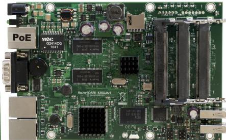
Five miniPCI slots and three Gigabit Ethernet ports give you enough connectivity options to use the RB435G as the central part of your network. Now with Gigabit ports, to properly utilize all the speed 802.11n with Nv2 wireless.
