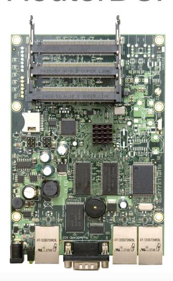
The RB433AH is a more powerful version of the standard RB433. The 128MB DDR will be capable of supporting new RouterOS features coming. The microSD slot supports an additional memory card that can be used for a Dude database and other features.
