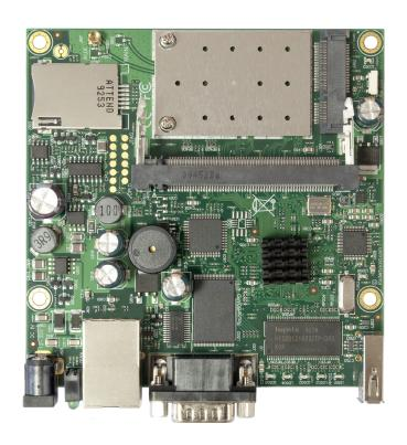
The RB411UAHR has it all, just as the name suggests. It has the popular high-speed CPU, a miniPCI-e slot and a SIM slot for 3G modems, a USB 2.0 port for attaching external storage, a regular miniPCI card slot for 802.11abgn wireless cards, a Ethernet port and a built-in wireless radio.
