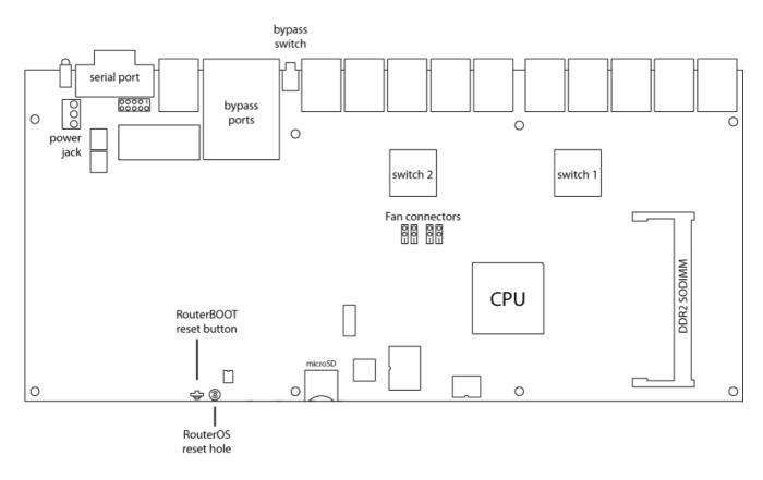
You can download the board dimensions and case design files (PDF and DXF) from <u>www.routerboard.com</u>
